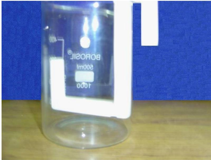
Figure 2.6: Arrangement showing the nanorod growth in a solution. The seeded substrates were kept upside down at the bottom of the tefflon stand dipped into the solution.
