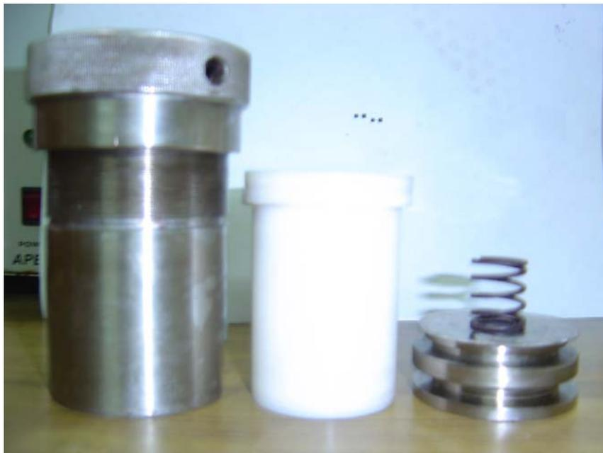
Figure 2.2: Autoclave used for high pressure synthesis. The teflon beaker and the steel plates are parts of this autoclave
