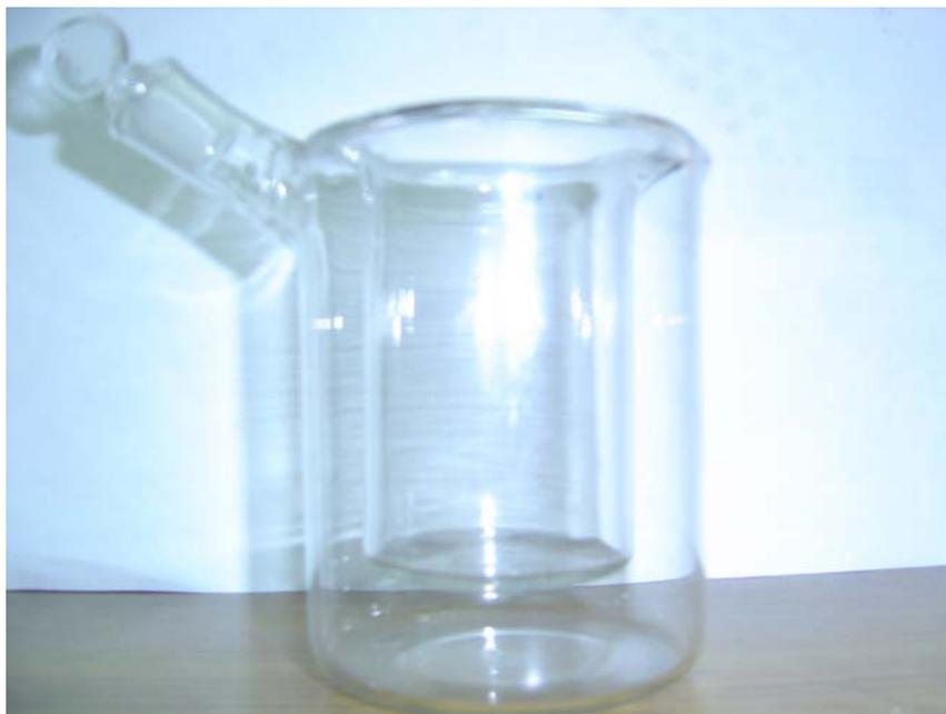
Figure 2.1: The specially designed temperature bath used for uniform heating during solution growth of ZnO nanostructures. The outer cylindrical shell contains a liquid like water or oil to maintain a uniform temperature all through the sample column.
